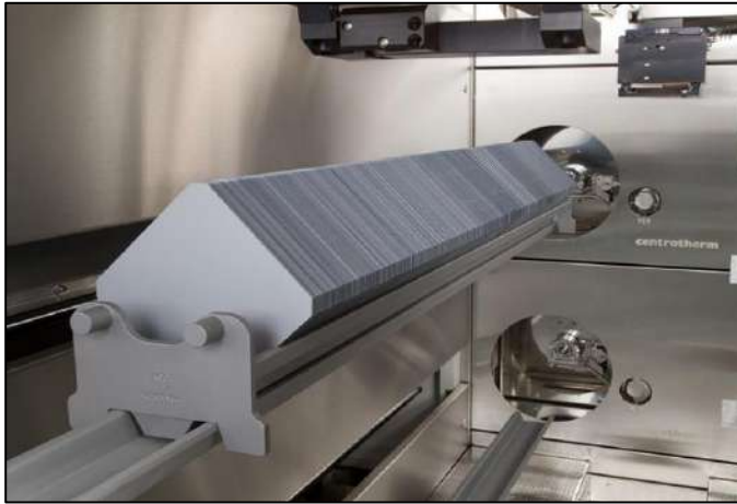
High-capacity diffusion boot with back-to-back loaded wafers
